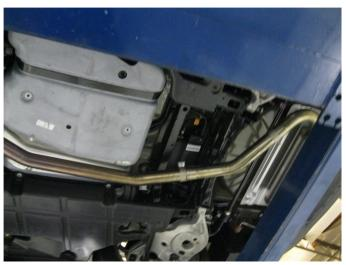
**Step 4.** Loosely install the Mid Pipe to the Resonater Assembly and Connecting Pipe using the supplied 2.50" clamps.
