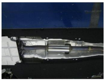
**Step 3.** Begin installing your new system by loosely attaching the inlet flange of the Resonator Assembly to the catalytic converter outlet using the OEM fasteners.
