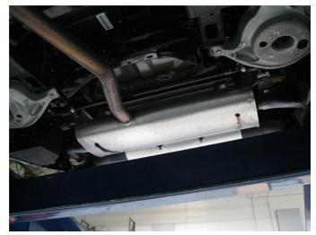
**Step 2.** Disengage the welded hangers from the rubber insulators on the muffler assembly. Again, retain all mounting hardware as it will be needed to mount your new system. The OEM exhaust may now be removed in one piece.
