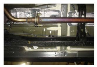
**Step 1.** Begin removal of the OEM exhaust system by unbolting the two spring loaded bolts attaching the exhaust to the catalytic converter. Do not discard or damage the OEM fasteners or rubber insulators as they will be used to install the new system.
