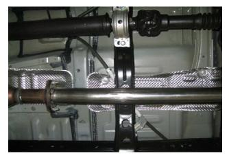
**Step 3.** Begin installation of your new MAGNAFLOW system by attaching the Inlet Pipe Assembly to the catalytic converter outlet using the OEM fasteners and insulator. Keep all fasteners and clamps loose until final adjustment.
