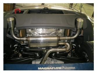
**Step 5.** Next use the supplied 2.50" clamps to attach the Muffler Assembly to the Mid Pipe and the Tail Pipe Assemblies to the Muffler. Fit hangers into rubber insulators.
