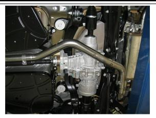
**Step 4.** Next use the supplied 2.50" clamp to attach the Mid-Pipe to the Resonator Assembly.
