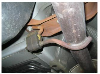
**Step 1.** begin removal of the OEM system by loosening the clamp at the outlet the flex pipe. Working front to rear detach all hangers from rubber insulators and remove the system. Retain rubber insulators as they will be re-used the mount the new system.
