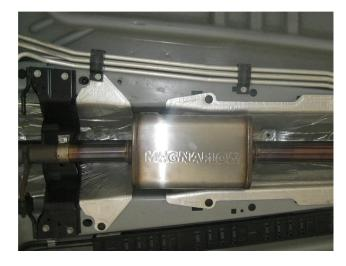
**Step 2.** Begin installation of the new system by fastening the Resonator Assembly to the outlet of the flex pipe using the supplied 2.25" clamp.
