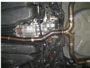
**Step 3.** Next attach the Mid-Pipe Assembly to the Resonator, followed by the Y-Pipe Assembly. Use supplied 2.50" clamps and fit hangers into rubber insulators.
