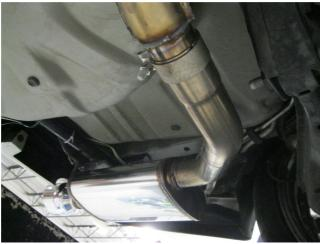
**Step 4.** Finish by installing both Muffler Assemblies using the supplied 2.50" clamps, fitting the hangers into the rubber insulators.
