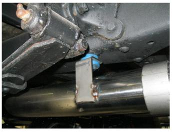
**Step 4.** The welded bracket on each Over Axle Pipe needs to be attached to the chassis also. A hole will have to be drilled to locate the supplied mounting hardware and rubber grommet as shown.
