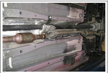
**Step 1.** to remove the OEM exhaust system, unbolt the clamp at the catalytic converter. Disengage the welded hangers from the rubber isolators and remove the complete exhaust system.
