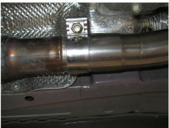
**Step 2.** Begin installation of your new system by fitting the Inlet Pipe Assembly to the catalytic converter outlet. Locate the welded hanger to the rubber isolator. Secure using the supplied clamp. Leave all clamps loose for final adjustment.
