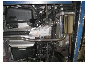
**Step 3.** Install the Mid Pipe, Muffler and Tail Pipe Assemblies in a similar fashion.
