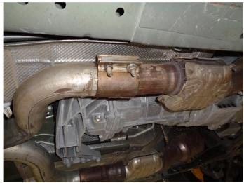
**Step 1.** To remove the OEM exhaust system you will first need to loosen the clamps attaching the exhaust system to the catalytic converter outlet pipes. Working front to rear disengage all welded hangers from the rubber insulators. The OEM exhaust system can now be removed. Retain all mounting hardware as it will be needed to install your new MAGNAFLOW system.
