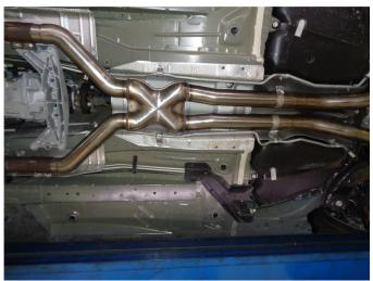
**Step 2.** Begin installing the new system by loosely attaching both inlet pipes of the X-Pipe Assembly to the catalytic converter outlets using the OEM clamps.
