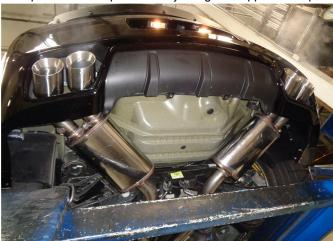
**Step 4.** Loosely install both muffler assemblies using the supplied clamps. Locate all welded hangers to the OEM rubber insulators.
