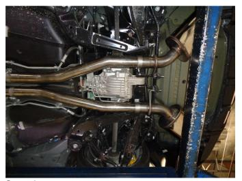
**Step 3.** Next, loosely install both driver and passengers side Mid Pipes to the X-Pipe Assembly using the supplied clamps.
