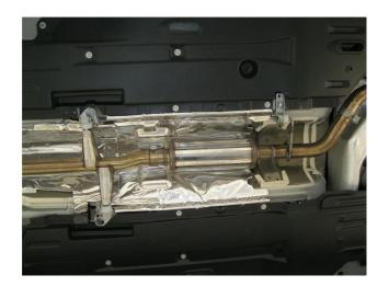
**Step 2.** To install the new Magnaflow exhaust system begin by attaching the Resonator Assembly to the outlet of the OEM system using a supplied 2.50" clamp and fitting the hanger into the rubber insulator. Leave all clamps loose until final adjustment of the system.
