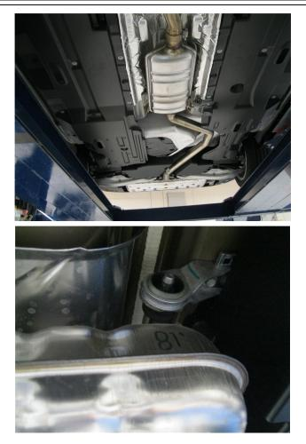
**Step 1.** Begin removal of the OEM exhaust by loosening the clamps located in front of the factory resonator and muffller assemblies. Working front to rear, disengage the hangers from the rubber insulators and remove the system. On this vehicle it may be easier to un-bolt the insulators from the frame rails. Do not damage or discard the rubber insulators as they will be re-used to install the new Magnaflow system.
