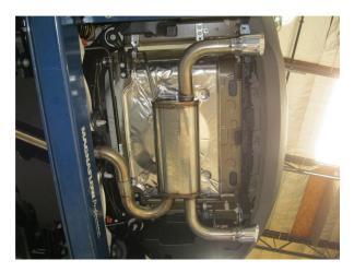
**Step 4.** Complete the installation by attaching the Muffler Assembly to the Mid-Pipe using a 2.50" clamp and fitting the hangers into the rubber insulators.
