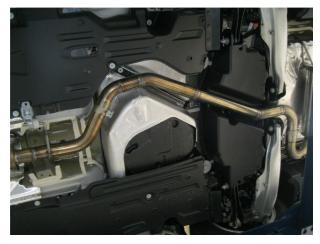
**Step 3.** Next attach the Mid-Pipe to the Resonator Assembly using a 2.50" clamp.
