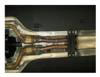
**Step 2.** Begin installation of the new system by fastening the Resonator Assembly inlets to the catalytic converter using the OEM fasteners and supplied gaskets (Leave all clamps and fasteners loose for final adjustment of the complete system.)
