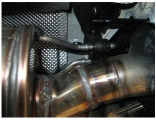
**Step 3.** Next Install the Mid-Pipe Assemblies to the outlets of the Resonator Assembly and then the Muffler Assemblies to the Mid-Pipes using the supplied 2.50" clamps. Insert hangers into rubber insulators. Re-attach brace.
