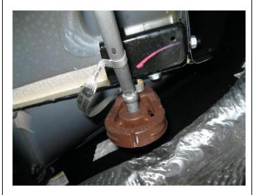
**Step 1.** To remove the OEM exhaust system loosen the clamp fastening the Y-Pipe/Muffler Assembly to the Catalytic Converter outlet, un-clip the ground strap from the rear hanger. Disengage the hangers from the rubber insulators and remove the system. Do not discard the or damage the rubber insulators as they will be used to mount the new system.
