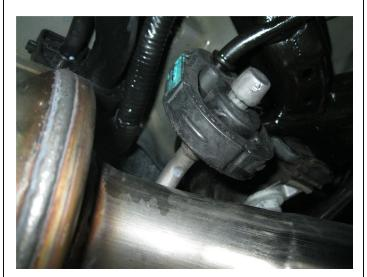
**Step 4.** Finish by installing both Tail Pipe Assemblies using the supplied 2.25" clamps, fitting the hangers into the rubber insulators and re-attaching ground strap..
