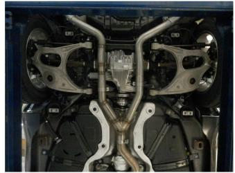
**Step 3.** Next attach the driver and passenger side Extension Pipes using the supplied 2.25" clamps.
