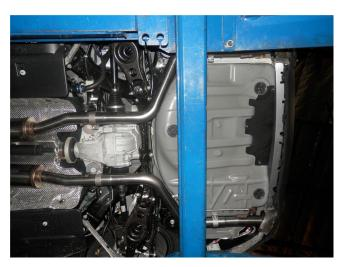
**Step 3.** Attach the Mid-pipes to the Resonator Assembly with supplied 2.50 Clamps and fit hangers into rubber insulators. Remember to re-attach the ground strap to the hanger. Finish the installation by mounting the Tailpipe Assemblies to the Mid-pipes with supplied clamps and aligning them with the openings in the rear valance and mounting underbody braces.
