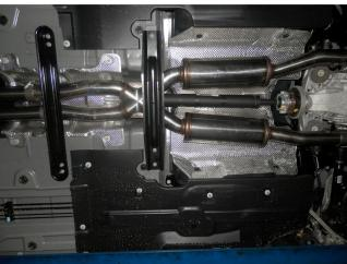
**Step 2.** Begin installation of the new system by attaching the Driver and Passenger side (Passenger is the longer of the two pipes) inlet pipes to the outlets of the OEM system using the supplied 2.50" clamps. Next attach the Resonator Assembly to the inlet pipes with supplied clamps and insert the hangers into the rubber insulators.
