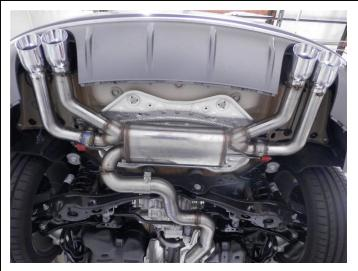
**Step 6.** Loosely install the Muffler Assembly using the supplied clamp. Attach the welded hangers to the rubber insulators. Re-attach both electrical connectors to the exhaust valve motors.
