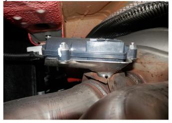
**Step 3.** Once the OEM system has been removed undo three nuts attaching each exhaust valve motor to the valve and remove.
