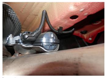
**Step 1.** To remove the OEM exhaust system you will first need to unplug the exhaust valve control motors located on the OEM muffler assembly. Unbolt and remove the OEM cross-member.
