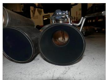
**Step 4.** Before installing your new exhaust system attach the OEM valve motors to each valve using the OEM hardware. The alignment spring on the motor will need to be engaged into the keyway slot of the new valves.
