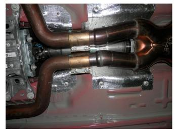
**Step 5.** Install the X-Pipe Assembly to the OEM slip clamp. Engage the welded hangers to the rubber insulators. Leave all clamps loose for final adjustment of the system.
