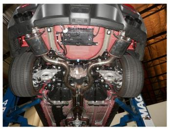
**Step 7.** Loosely install the Muffler Assemblies using the supplied clamp. Attach the welded hangers to the rubber insulators. Re-attach both electrical connectors to the exhaust valve motors.
