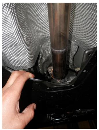
**Step 3.** Begin installation of your new MAGNAFLOW system by attaching the Inlet flange of the Inlet Resonator Assembly to the catalytic converter outlet using the OEM fasteners. Engage the welded hanger to the rubber isolator. Keep all fasteners and clamps loose until final adjustment.
