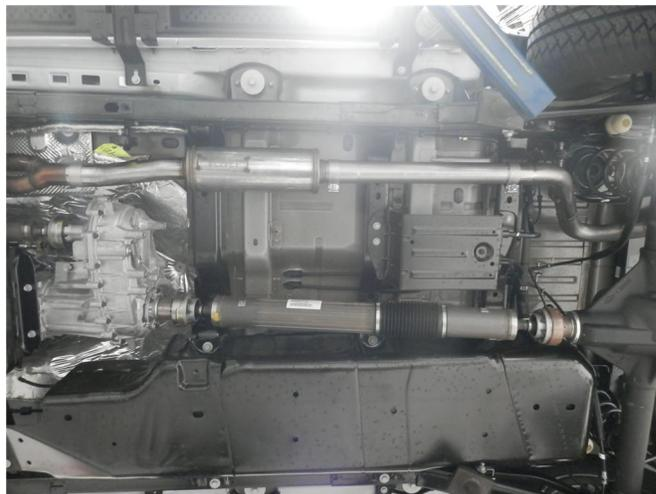
**Step 4.** The included Extension Pipe is required for the four door model only. It is to be installed between the Resonator Assembly and the Over-Axle Pipe Assembly. If you have the two door this pipe may be discarded.
