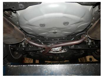
**Step 2.** Next, remove both muffler assemblies by unbolting them from OEM Y-Pipe assembly. Remove all welded hangers from the rubber insulators. The exhaust system may now be removed. Retain all mounting hardware as it will be needed to install your new MAGNAFLOW system.
