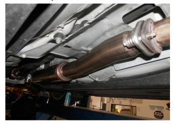
**Step 3.** Begin installation of the new system by fastening the Inlet Pipe Assembly to the outlet of the catalytic converter using the OEM hardware.
