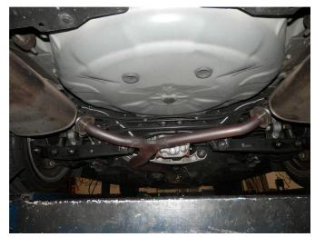
**Step1.** Remove both muffler assemblies by unbolting them from OEM Y-Pipe assembly. Remove all welded hangers from the rubber insulators. The exhaust system may now be removed. Retain all mounting hardware as it will be needed to install your new MAGNAFLOW system.
