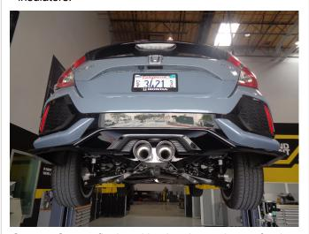
Step 5: Once a final position has been chosen for the new exhaust system, evenly tihgten all clamps from front to rear using the torque specifications on page one of these instructions. Inspect all fasteners after 25-50 miles for operation and re-tighten if necessary.
