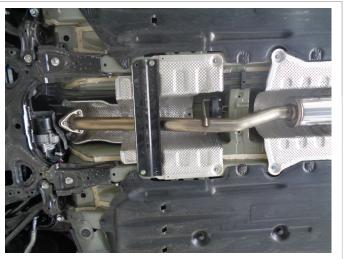
Step 2: Begin installing your new system by loosely bolting both inlet flange of the Resonator Assemblies to the catalytic converter outlets using the OEM hardware. Engage the welded hangers to the rubber insulator.
