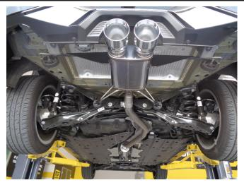
Step 4: Finish by loosely installing the Muffler Assembly to the Mid Extension pipes using the supplied clamp and fitting the hangers into the rubber insulators.
