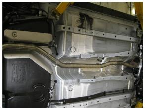
**Step 3.** Begin installation of your new MAGNAFLOW system by attaching the Inlet Pipe Assembly to the catalytic converter outlet using the 2.25" supplied Clamp and OEM insulator. Keep all fasteners and clamps loose until final adjustment.
