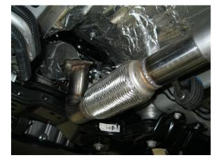
**Step 2.** You are now ready to install your new MAGNAFLOW system. Attach the the Inlet Pipe Assembly to the OEM catalytic converter outlet using the OEM hardware. Engage the welded hanger to the OEM rubber insulator (Leave all clamps and hardware loose for final adjustment of the complete system).
