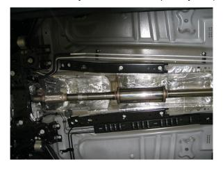
**Step 3.** Next slip the Resonator Assembly inlet pipe on to the outlet of the Inlet Pipe Assembly and loosely secure using the supplied 2.25" clamp and 15mm socket. Engage welded hanger to the OEM rubber insulator.
