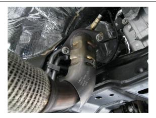
**Step 1.** Begin removing the OEM exhaust by unbolting the OEM inlet flange at the outlet of the OEM catalytic converter with a 13mm socket. Remove the welded hangers from the rubber insulators using a pry bar. Do not discard or damage the insulators or the flange fasteners as they will be needed to install your new system. The OEM system may now be removed.
