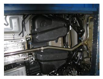
**Step 4.** Slip the inlet of the Y-Pipe Assembly over the outlet of the Resonator Assembly and loosely secure using the supplied 2.50" clamp and 15mm socket. Engage all welded hangers to the OEM rubber insulators. Install the Muffler Assemblies using a similar procedure.
