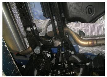
**Step 2.** To remove the OEM system you will need to cut the exhaust pipe at the over axle pipe. Disengage all welded hangers from the rubber isolators. the exhaust can now be removed. Retain all fasteners and insulators as the will be needed to mount your new MAGNAFLOW system.
