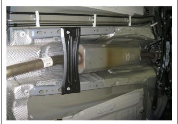
**Step 1.** Remove the OEM system by first unbolting the two nuts at the flange attaching the stock inlet pipe to the catalytic converter.
