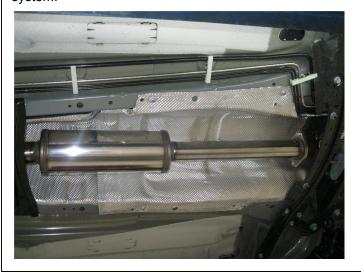
**Step 3.** Install your new system by first attaching the Inlet Resonator Assembly to the catalytic converter outlet using the supplied hardware.
