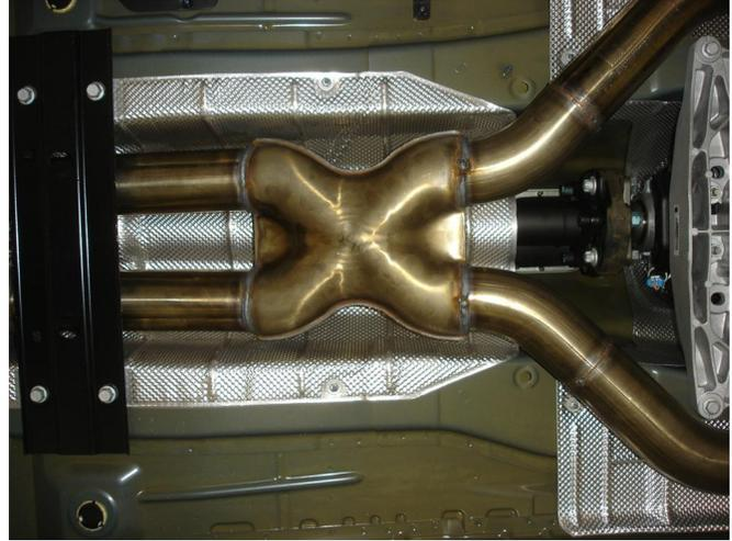
**Step 2.** Begin installation of the new system by loosely attaching the X-Pipe Assembly to the catalytic converter outlets using the OEM clamps.
