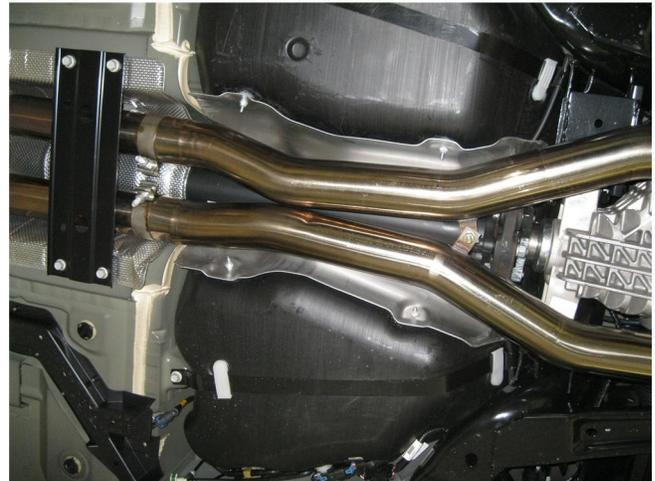
**Step 3.** Next attach the Mid Pipe Assemblies to the X-Pipe using the supplied 3.00" clamps. Loosely connect the Mid Pipes using the supplied 3/8 fasteners at the brackets. The D/S bracket should be on top of the P/S bracket per the photo. .
