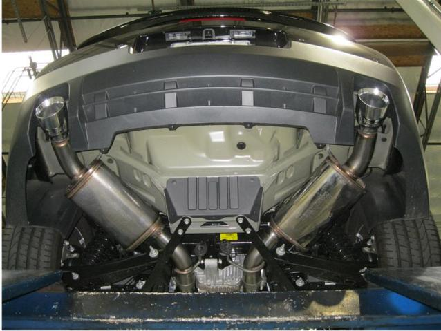
**Step 4.** Next attach the driver and passenger side Muffler Assemblies to the Mid Pipe Assemblies using the supplied 3.00" clamps and by fitting the hangers into the rubber insulators. Complete the installation by re-installing all the braces that were removed.
