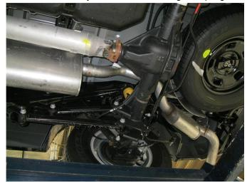
**Step 2.** Next unbolt the OEM clamp attaching the tail pipe assembly to the muffler assembly. Remove the welded hangers from the rubber insulators using a pry bar. Do not discard or damage the insulators as they will be needed to install your new system. The OEM system may now be removed.
