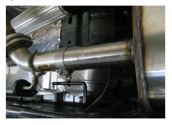
**Step 3.** You are now ready to install your new MAGNAFLOW system. Loosely attach the the Muffler Assembly to the OEM pipe outlet using the supplied 3.00" clamp. Engage the welded hanger to the OEM rubber insulator. Leave all clamps and hardware loose for final adjustment of the complete system.
