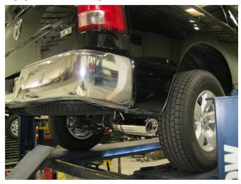
**Step 5.** Once a final position has been chosen for the new system, evenly tighten all fasteners from front to rear using the torque specifications on page one of this document. Inspect all fasteners after 25-50 miles of operation and retighten if necessary.
