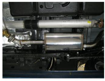
**Step 4.** Slip the inlet of the Tail Pipe Assembly over the outlet of the Muffler Pipe Assembly and loosely secure using the supplied 3.00" clamp and 15mm socket. Engage all welded hangers to the OEM rubber insulators.
