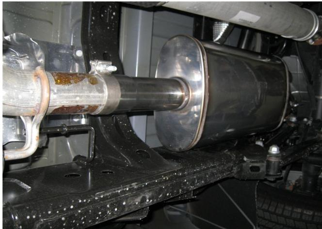
**Step 4.** Install the supplied hanger assembly using a pre drilled hole in the drivers side sub frame and the supplied hardware. This will be used with the supplied rubber insulator to locate the new drivers side Mid Pipe Assembly hanger. Slip the inlet of both Mid Pipes over the outlet of the Muffler Assembly and loosely secure using the supplied 2.50" clamp and 15mm socket. Engage all welded hangers to the OEM rubber insulators.
