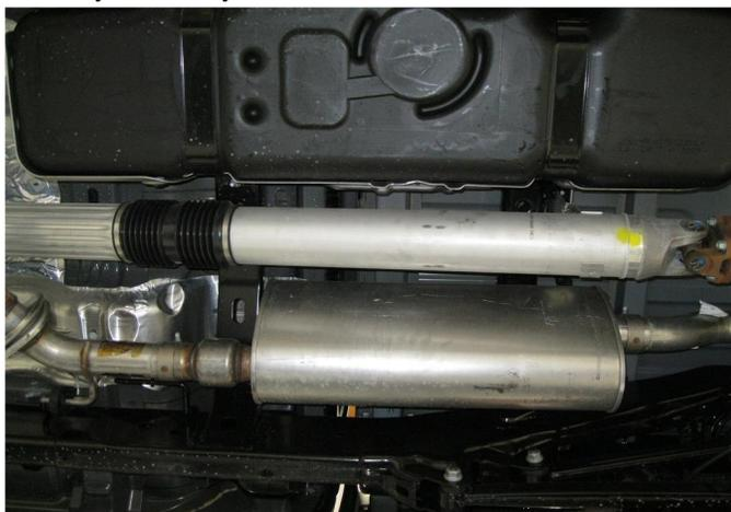
**Step 3.** You are now ready to install your new MAGNAFLOW system. Loosely attach the the Muffler Assembly to the OEM pipe outlet using the supplied 3.00" clamp. Be sure to line up the large notch in the pipe with the alignment peg. Engage the welded hanger to the OEM rubber insulator. Leave all clamps and hardware loose for final adjustment of the complete system.
