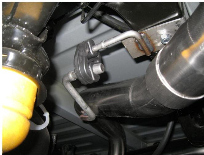
**Step 5.** Install both Tail Pipe Assemblies in a similar fashion. Use the supplied rubber Insulator to locate the drivers side welded hanger.
