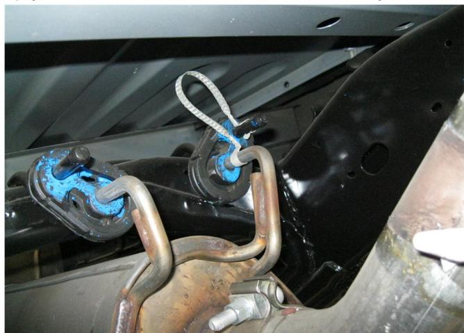
**Step 2.** Next unbolt the OEM clamp attaching the inlet muffler assembly to the outlet pipe of the flange coupling. Remove the welded hangers from the rubber insulators using a pry bar. Do not discard or damage the insulators as they will be needed to install your new system. There is a grounding strap that needs to be unclipped. The OEM system may now be removed.
