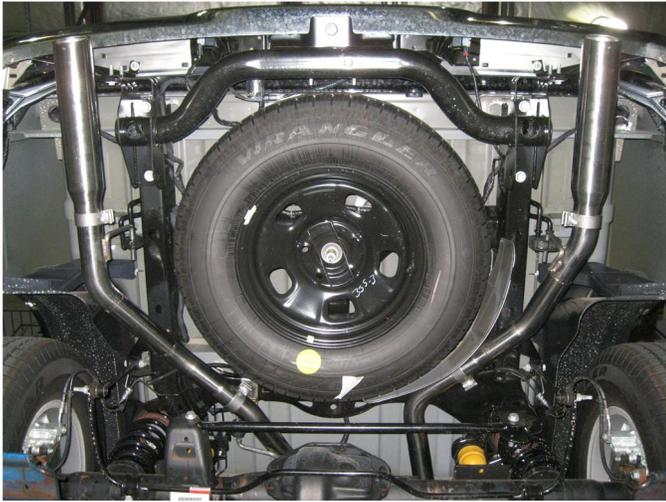
**Step 6.** Loosely attach the polished tips using the supplied 2.50" clamps to the desired position.
