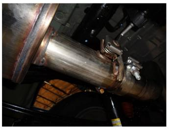
**Step 4.** Next loosely attach the Tail Pipe Assembly to the valve outlet on the Muffler Assembly using the supplied clamp. Engage the welded hanger to the rubber insulator.
