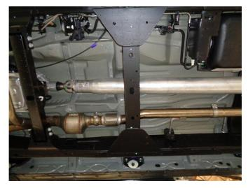
**Step 2.** Begin installation by loosely attaching the Inlet Pipe Assembly to the catalytic converter ball flare using the OEM hardware. Engage the welded hanger to the rubber insulator.
