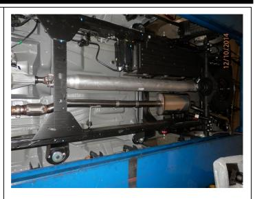
**Step 3.** Crew Cab Short Bed vehicles only will require the 12.5" Extension Pipe to be fitted between the Inlet Pipe Assembly and the Muffler Assembly. Loosely attach the Muffler Assembly using the supplied clamps. Engage all welded hangers to the rubber insulators.
