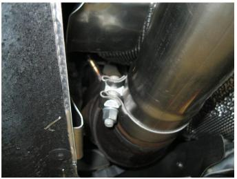
**Step 2.** Begin installation of the new system by fastening the inlet Y-Pipe Assembly to the outlet of the catalytic converter using the OEM band clamp.
