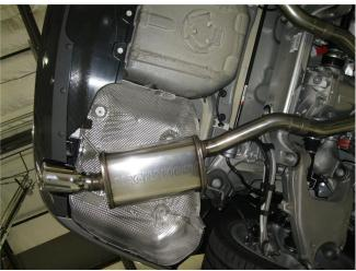
**Step 4.** Finish by installing both Muffler Assemblies using the supplied clamps, fitting the hangers into the rubber insulators and re-attaching the cross brace.
