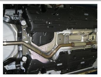
**Step 4.** Next use the supplied 2.50" clamp to attach the Mid-Pipe to the Resonator Assembly.
