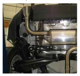
**Step 5.** Next use the supplied 2.50" clamps to attach the Muffler Assembly to the Mid Pipe and the Tail Pipe Assemblies to the Muffler. Fit hangers into rubber insulators.
