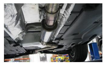
**Step 3.** Begin installation of your new MAGNAFLOW system by attaching the Resonator Assembly to the "Y" collector outlet using the supplied 2.50" clamp. Keep all fasteners and clamps loose until final adjustment.
