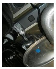
**Step 2.** Disengage hangers from rubber insulators and remove the OEM exhaust.
