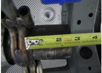
**Step 1.** Removal of this exhaust system requires cutting and de-burring the pipe 2.50" behind the hanger assembly welded to the pipe behind the catalytic converter. To accomplish this you must remove the cross brace and catalytic converter shield.
