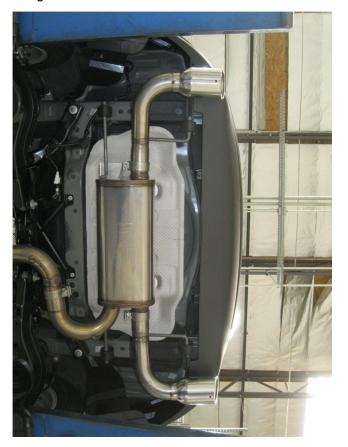
**Step 5.** Finish by attaching the Tail Pipe Assemblies to the Muffler with the supplied 2.50" clamps and fit hangers into rubber insulators.
