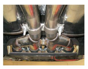
**Step 6.** Once a final position has been chosen for the new exhaust system, evenly tighten all clamps from front to rear using the torque specifications on page one of the instructions. Inspect all fasteners after 25-50 miles of operation and re-tighten if necessary. the Muffler assemblies using the provided 2.50" clamps.
