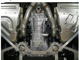
**Step 3.** Next, Loosely attach the Muffler Assemblies to the Inlet pipe using the provided 3.00" clamps. You will then need to fasten the provided cross bracket in place between the two muffler assembles using the provided 1/4" fasteners. Insert all hangers in the rubber isolators.
