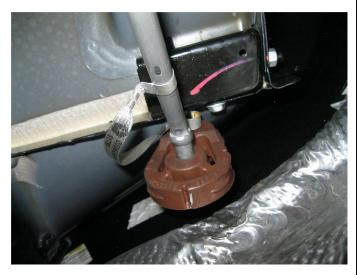
**Step 1.** To remove the OEM exhaust system loosen the clamp fastening the Y-Pipe/Muffler Assembly to the Catalytic Converter outlet, un-clip the ground strap from the rear hanger. Disengage the hangers from the rubber insulators and remove the system. Do not discard the or damage the rubber insulators as they will be used to mount the new system.
