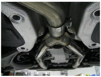
**Step 2.** Begin installation of the new system by fastening the inlet Y-Pipe Assembly to the outlet of the catalytic converter using the supplied 2.75" band clamp. Leave all clamps loose for the final adjustment of the complete system.
