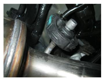
**Step 4.** Finish by installing both Muffler Assemblies using the supplied 2.25" clamps, fitting the hangers into the rubber insulators and re-attaching ground strap..
