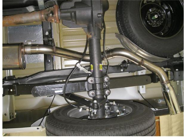
**Step 3.** Finish by installing the Tail Pipe Assembly to the Tail Pipe Extension using the supplied 3.00" clamp, fitting the welded hanger into rubber insulator.
