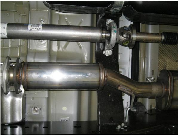
**Step 2.** To begin, fasten the Inlet pipe assembly to the catalytic converter using the provided 10mm nuts, the OEM clamp assembly and by fitting the welded hanger into the OEM rubber insulator (Leave all clamps and fasteners loose for final adjustment of the complete system.) Install the Muffler to the Inlet Pipe Assembly using the supplied 3.00" clamp. Next install the Tailpipe Extension to the Muffler in the similar fashion using the supplied 3.00" clamp.
