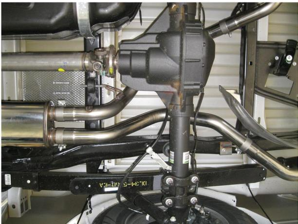
**Step 2.** Begin by fastening the Resonator Assembly to the catalytic converter using the supplied 10mm nuts, the OEM clamp assembly and by fitting the welded hanger into the OEM rubber insulator (Leave all clamps and fasteners loose for final adjustment of the complete system.) Install the Muffer to the Resonator Assembly using the supplied 3.00" clamp. Next install the Tailpipe Extensions to the Muffer in the similar fashion using the supplied 2.50" clamps.
