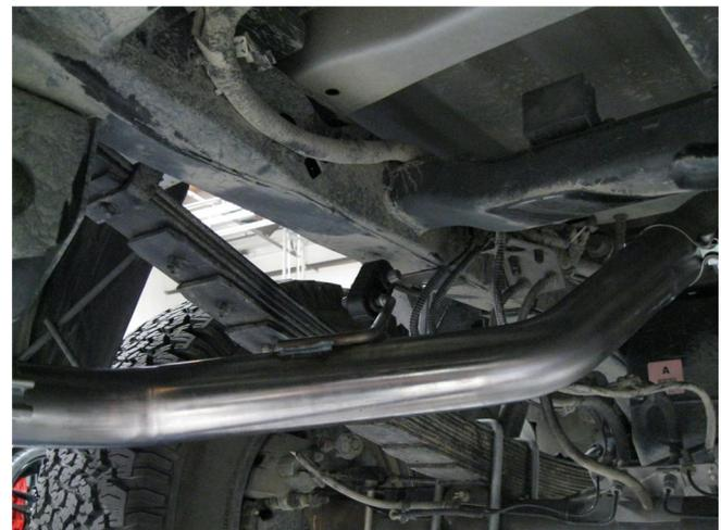
**Step 3.** Next you will need to use the supplied U-Clip nut and attach them to the receiving cut outs in the bottom of the frame member. Fasten the supplied hanger assemblies to the frame members using the supplied bolts on both the Driver and Passenger side. Then install the Tail Pipe Assemblies to the Tail Pipe Extensions using the supplied 2.50" clamp, fitting the welded hangers into rubber insulators.
