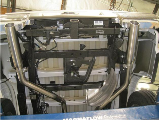
**Step 4.** Lastly, install the tips to the Tail pipe Assemblies using the supplied 2.50" clamps. The supplied adjustable tips are design to fit a variety of aftermarket bumpers and rollpans, once a position is decided for the tips it is recommended to have them welded into place.
