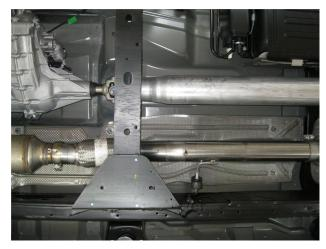
**Step 2.** To begin, fasten the Inlet pipe assembly to the catalytic converter using the OEM clamp assembly and by fitting the welded hanger into the OEM rubber insulator (Leave all clamps and fasteners loose for final adjustment of the complete system.)
