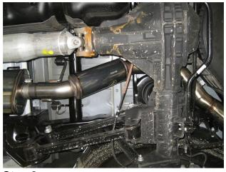
**Step 2.** Begin by attaching the Muffler Assembly to the factory outlet and the Resonator Assembly to the Muffler Assembly outlet using the supplied 3.50" clamps. Fit the hangers into the rubber insualtors. Leave all clamps loose until final adjustment.
