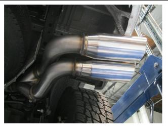
**Step 3.** Next Install the Tail Pipe Assembly using the supplied 4.00" clamp and fit the welded hanger into the rubber insulator.
