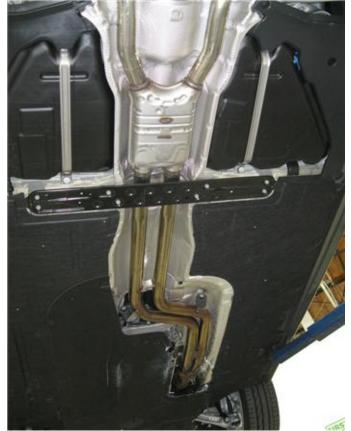
**Step 1.** To allow for extraction of the OEM system you must first remove the underside cross brace. Next loosen the clamp at the outlet of the catalytic converter. Working front to rear detach all hangers from rubber insulators and remove the system. Retain rubber insulators and clamp as they will be re-used the mount the new system.
