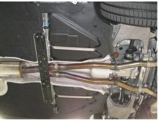
**Step 3.** Next attach the Resonator Assembly to the Y-Pipe Assembly followed by the two Mid-Pipe assemblies, use supplied clamps and fit hangers into rubber insulators.
