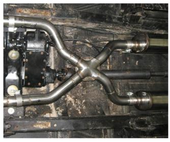
**Step 1.** After removal of the OEM system you can begin installation of the Magnaflow system. Start by attaching the X-Pipe Assembly to the factory outlets using the supplied 2.50" clamps. Leave all clamps and fasteners loose until final adjustment.
