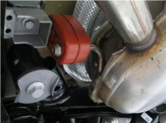
**Step 1.** Begin removal of the OEM system by loosening at the inlet of the Resonator and removing the black tubular cross brace. You can then disengage the welded hangers from the rubber insulators, working rearward finish removing the system. Do not damage or discard the rubber insulators or OEM clamp as they will be re-used to mount the new system.
