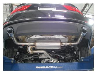
**Step 4.** Complete the installation by fastening the Driver and Passenger side Tailpipe Assemblies to the Muffler Assembly with the supplied 2.50" clamps and fit the hangers into the insulators. Re-install the factory brace.
