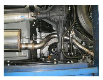
**Step 3.** Complete the initial installation by attaching the Extension Pipe Assembly (containing the exhaust valve) to the Muffler and the Resonator/Tailpipe Assembly the Extension Pipe using the suplied 3.00" clamps.
