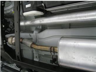
**Step 1.** To remove the OEM exhaust system, you will first need to cut the pipe behind the muffler before it goes over the axle. You can then disengage the welded hangers from the rubber insulators and remove the tailpipe. Unfasten the muffler inlet from the catalytic converter at the clamp junction. Do not damage or discard the OEM fasteners or rubber insulators, as they will be reused to mount the new system. Disengage the muffler hangers and remove it from the vehicle.
