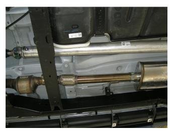
**Step 2.** Begin installation of the new system by attaching Inlet Pipe Assembly at the ball flare using the OEM clamp and fitting the hanger into the rubber insulator. Next attach the muffler to the inlet pipe using a supplied 3.00" clamp. Leave all clamps loose for final adjustment of the complete system.
