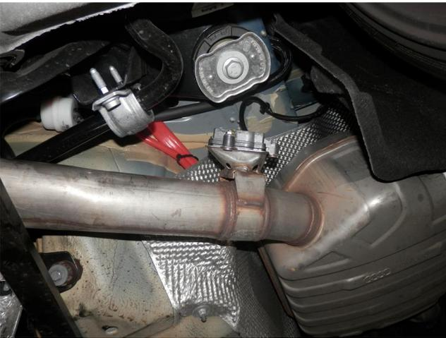
**Step 1.** To remove the OEM exhaust system you will need to remove the cross braces/stiffener and unplug the electronic exhaust control valves at the rear of the vehicle . Start by loosening the clamps at the catalytic converter junctions, working rearward disengage the hangers from the rubber insulators (retain rubber insulators and OEM clamps) and remove the system.
