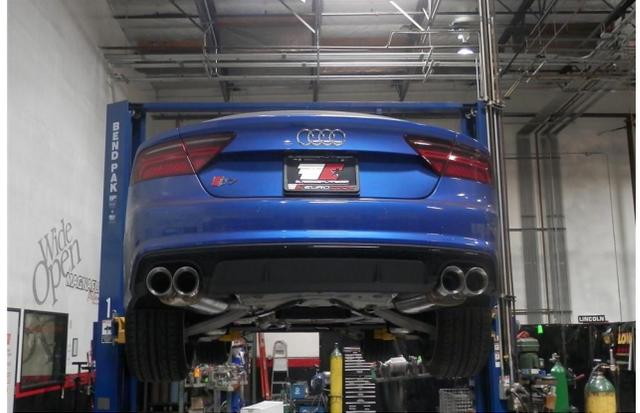
**Step 6.** Once a final position has been chosen for the new exhaust system, evenly tighten all clamps from front to rear using the torque specifications on page one of the instructions. Inspect all fasteners after 25-50 miles of operation and re-tighten if necessary.
