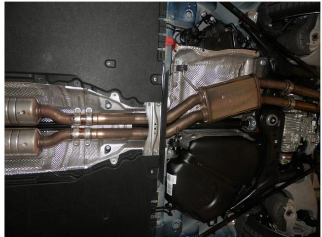
**Step 3.** Begin installation of the new system by fastening the Resonator Assembly inlets to the catalytic converters using the OEM clamps and fitting the hangers into the rubber insulators (Leave all clamps and fasteners loose for final adjustment of the complete system.)
