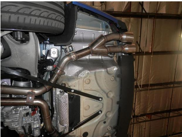
**Step 5.** Finish by installing the Tailpipe Assemblies to the outlets of the Mid Pipes using the supplied V-Band clamps. Insert hangers into rubber insulators and reattach valve motor connector plugs. Install braces.
