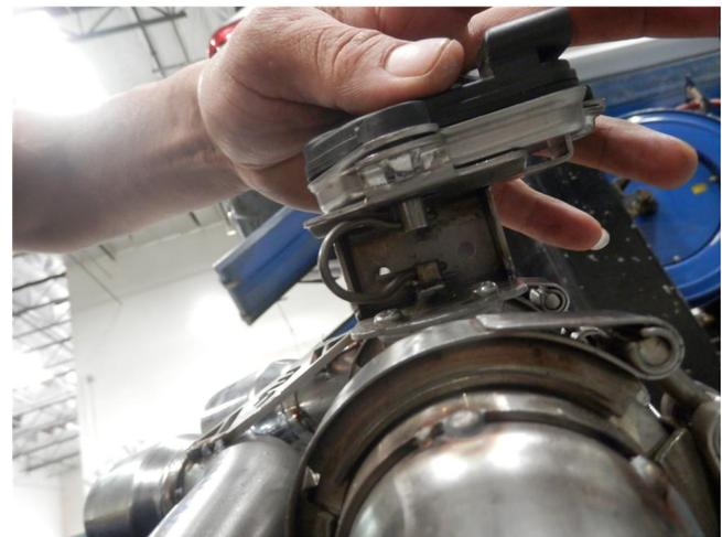
**Step 4.** At this point the OEM exhaust control valve motor can be bolted to the valve assembly on the new Muffler Assembly. Align the keyways in the valve motor and shaft of the new valve. Mate both keyway notches using the OEM indexing spring. Secure the valve motor using the three supplied mounting bolts. **\*\*NOTE: Do NOT loosen or undo the V-Band Clamps, they are designed for one time use only. Once the clamp is tightened it can not be reused.**
