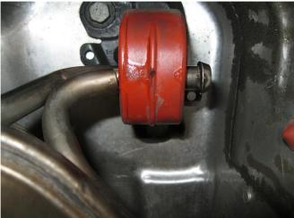
**Step 1.** Begn removal of the OEM exhaust by loosening the clamp located behind the catalytic converter. Do not damage or discard the clamp or rubber insulators as they will be used to install your new system. Disengage the hangers from the rubber insulators and remove the OEM exhaust.
