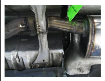
**Step 2.** Begin installation of the new system by fastening the Muffler Assembly to the outlet of the catalytic converter using the OEM clamp and inserting the hangers into the rubber insulators. Leave clamps loose until final adjustment of the exhaust.
