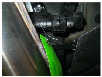
**Step 3.** Next attach the Tailpipe Assembly to the Muffler Assembly using the supplied 3.00" clamp and fit the hanger into the rubber insulator.
