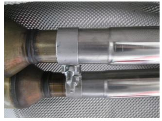
**Step 2.** Begin installation of the new system by slipping the inlet ends of the inlet muffler assembly over the pipes at the catalytic converter that you have just cut. Loosely secure with the supplied clamps.
