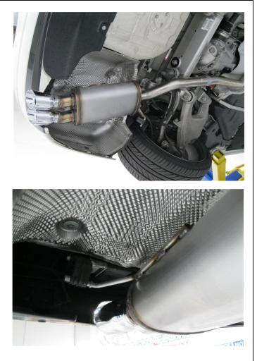
**Step 3.** Next attach the Tail Pipe Muffler Assembly to the Inlet Muffler Assembly using supplied clamp and fit hangers into rubber insulators. Re attach cross brace.
