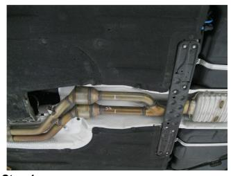
**Step 1.** To allow for extraction of the OEM system you must first remove the underside cross brace. Next cut the two pipes 3.25" behind the catalytic converter welds. Working front to rear detach all hangers from rubber insulators and remove the system. Retain rubber insulators and clamp as they will be re-used the mount the new system.
