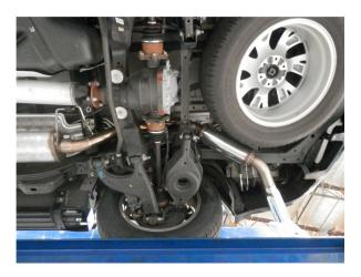
**Step 3.** Next Install the Mid pipe to the Resonator Assembly using a supplied 3.00" clamp. Complete the installation by attaching the Tailpipe / Muffler Assembly using the supplied 3.00" clamp and fit the welded hanger into the rubber insulator.
