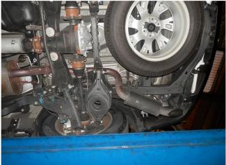
**Step 1.** To remove the OEM exhaust system begin by un-fastening the 2 bolt flanges at the catalytive converter outlets and behind the muffler. Next, working rearward with the exhaust supported disengage the hangers from the rubber insulators and remove the system. Do not damage or discard the rubber insulators or fasteners as they will be re-used to mount the new system.
