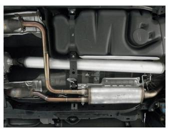
**Step 2.** Begin installation of the new system by attaching the Driver and Passenger side Inlet Assemblies to the catalytic converter outlets using the OEM fasteners and fitting the hangers into the rubber insulators. Next, Install the Resonator Assembly using the supplied 2.25" clamps and fit the welded hangers.
