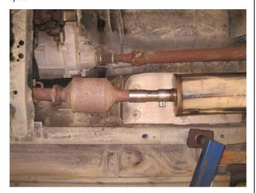
**Step 2.** Install the new system by attaching the new muffler assembly to the catalytic converter using the supplied 2.25" clamp and by locating the welded hanger to the rubber isolator. Be sure to align the locating notch in the muffler pipe with the indexing peg on the OEM system. Leave all clamps and fasteners loose for final adjustment of complete system.
