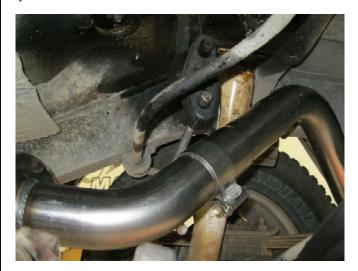
**Step 3.** Loosely attach the Tail Pipe Assembly using the supplied 2.50" clamp.
