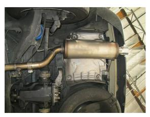
**Step 3.** Next Install the Muffler Assembly to the Inlet Pipe using the supplied 2.00" clamp. Insert hangers into rubber insulators.
