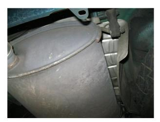
**Step 1.** To remove the OEM exhaust system begin by un-fastening the flange located behind the catalytic converter and disengaging all welded hangers from the rubber insulators. Do not damage or discard the rubber insulators or fasteners as they will be re-used to mount the new system. Working front to rear remove the exhaust from the vehicle.
