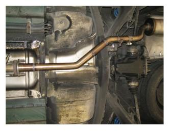
**Step 2.** Begin installation of the new system by fastening the Inlet Pipe Assembly to the catalytic converter outlet using the OEM fasteners and inserting the hanger into the rubber insulator (Leave all clamps and fasteners loose for final adjustment of the complete system).
