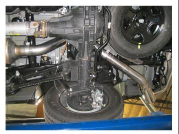
**Step 6.** Next Install the Tail Pipe Assembly in a similar fashion using the supplied 4.00" clamps and by fitting the welded hangers into the rubber insulators.
