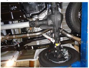
**Step 4.** Loosely install the Over Axle Pipe Assembly using the supplied clamp. Locate the welded hangers to the rubber insulators.
