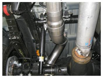
**Step 2.** Begin installation of the Magnaflow system by first clamping the 4"-5" Adapter Nipple to the newly cut outlet of the DPF using a supplied 4.00" clamp. Then attached the Over Axle Assy to the Adapter Nipple using the supplied 5" clamp and fitting the hangers in the rubber insulators (leave all clamps loose for final adjustment of the complete system). If your vehicle has an O2 sensor re-install at this time. If not, install the provided sensor boss plug.
