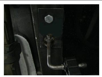
Step 7. For the Drivers Side Tail Pipe Assembly you will need to attach one of the supplied hangers. Bolt the supplied hanger bracket (shown) to the vehicles sub frame for year range '06 - '07. The threaded hanger is for year ranges '01 - '05. Both are mounted with the supplied hardware. Now engage the supplied hanger rubber to the newly mounted hanger and the welded hanger on the Tail Pipe Assembly.
