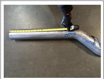
**Step 3.** The inlet end of the Mid Pipe Assembly may need to be trimmed depending on the year and cab configuration of your vehicle.
