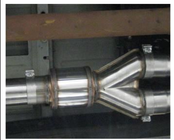
**Step 5.** Loosely Install the Muffler Assembly to the Extension Pipe Assembly using the supplied clamp. Engage all welded hangers to the rubber insulators.
