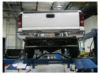
Step 8. Once a final position has been chosen for the new exhaust system, evenly tighten all clamps from front to rear using the torque specifications on page one of the instructions. Inspect all fasteners after 25-50 miles of operation and re-tighten if necessary.
